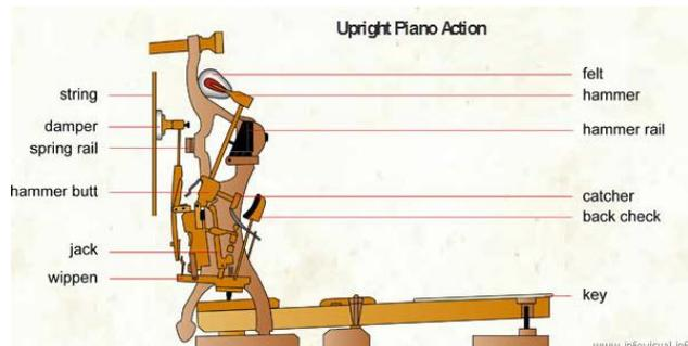
In fact there are 8 -10 adjustments per key that are made, totaling around 800. Some of these are set to a tolerance of .001 (a thousandth of an inch). Most pianos that we determine are "due for a regulation" are off by as much as 1/4" (.250). The fact that these pianos even function is pretty amazing, but what is really amazing is how much of an improvement the client notices once the regulation is completed.
